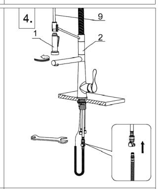
Connect the flexible hose(9) and spray head(1) to finish installation. Connect the inlet hoses to water supplies with fine sealing. Turn on the water supplies and check for leaks.
