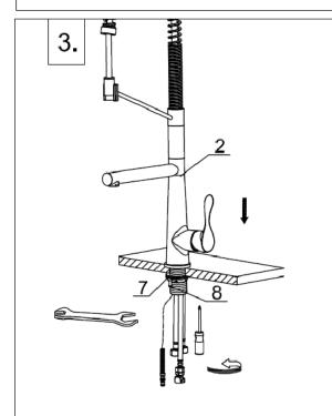
After adjusting the direction of the main body(2), tighten the edge nut(7) with hands and tighten the screws(8) with a Philips screwdriver.
