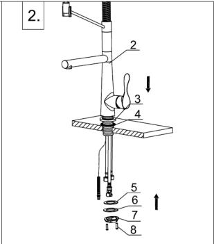
Make a faucet hole. Remove the screws (8), edged nut (7), metal gasket (6), and washer B (5) from the main body (2).
