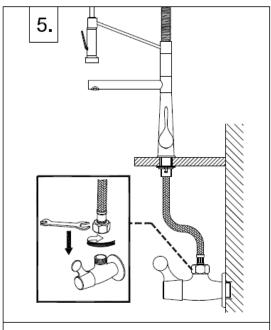
Connect the inlet hoses to water supplies with fine sealing. Turn on the water supplies and check for leaks.
